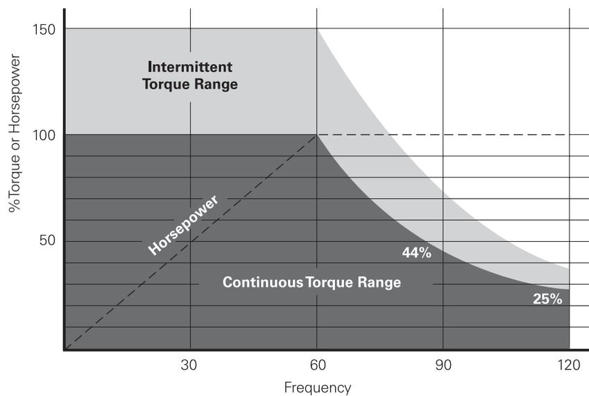
The sample motor described above is capable of operating at 100% rated torque continuously at low frequencies. Many motors are not capable of operating continuously at 100% continuous torque at low frequencies. Each motor must be evaluated before selecting it for use on an AC drive.
