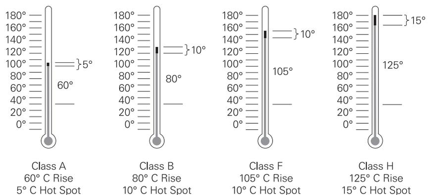
The operating temperature of a motor is important to efficient operation and long life. Operating a motor above the limits of the insulation class reduces the motor's life expectancy. A 10° C increase in the operating temperature can decrease the life expectancy of a motor as much as 50%.
