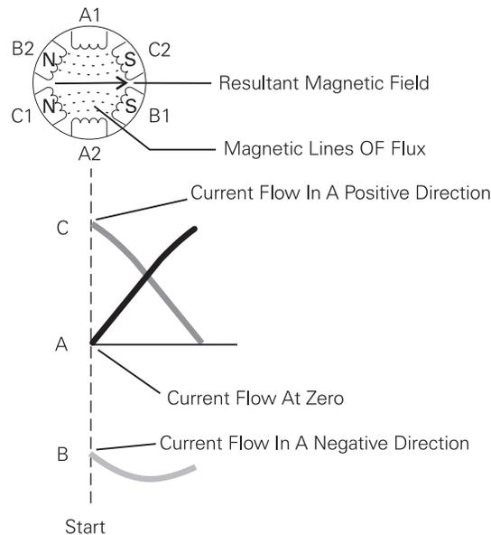
The amount of flux lines ( $\Phi$ ) the magnetic field produces is proportional to the voltage (E) divided by the frequency (F). Increasing the supply voltage increases the flux of the magnetic field. Decreasing the frequency increases the flux.
