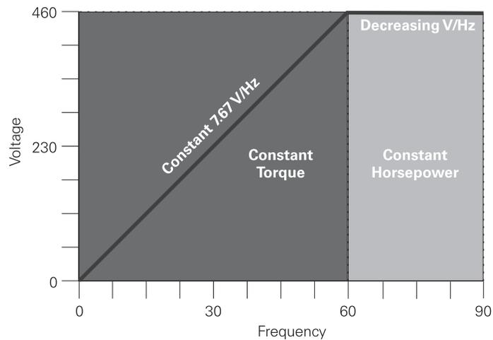
Horsepower remains constant as speed (N) increases and torque (T) decreases in proportion. The following formula applies to speed in revolutions per minute (RPM).
